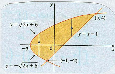
$$\iint_D xy \, dA = \int_{-3}^{-1} \int_{-\sqrt{2x+6}}^{\sqrt{2x+6}} xy \, dy \, dx$$
